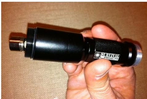
3. Carefully slide the heat sink holder over the driver assembly and thread it onto the battery compartment until fully seated. **Be careful not to twist or bend the driver leads excessively.** There will be some resistance to threading as the battery compartment o-ring is engaged into the heat sink holder during the last two threads.
