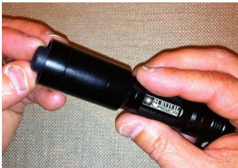
11. Place the lens cap over the lens when your laser is not in use. **CAUTION: Never** operate the laser with the lens cap in place. The cap will burn and combustion residue may be deposited onto the lens surface that can be extremely difficult to remove. **IMPORTANT: DO NOT** disassemble the laser once it is assembled. Doing so may break the wires connecting the driver to the diode and will invalidate your warranty.
