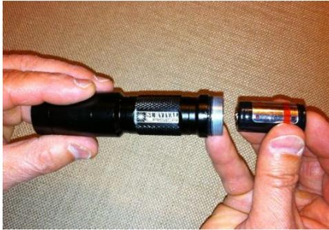
8. **WARNING:** Beginning at this step **put on your protective laser safety goggles** and ensure that anyone in the vicinity of your laser is wearing appropriate laser safety goggles. You must assume that your laser will begin functioning as soon as you screw on the tailcap. Install the batteries, **positive end first**, into the battery compartment.
