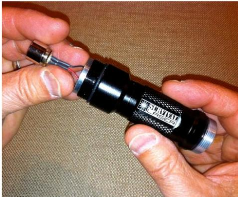
2. **CAUTION**: Remove any static charge on your body by touching a grounded metal object. Thread the diode & driver module into the battery compartment until fully seated. **Be careful not to twist or bend the driver leads excessively.**
