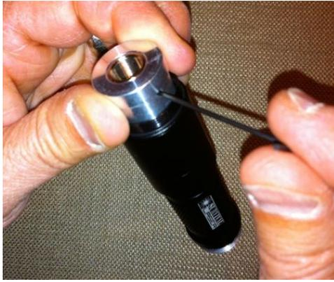
4. Slide the smaller diameter end of the heat sink over the exposed diode module on the diode & driver module assembly until the open end of the module is flush with the larger diameter end of the heat sink, then tighten the set screw **securely** against the module with the supplied Allen wrench. **Note:** If the set screw is not tightened sufficiently, the module could rotate while focusing the lens and break the driver wires or pull them off the diode.
