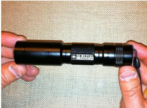
9. Point your laser in a safe direction, away from people, animals and highly flammable materials. Thread the tailcap w/switch onto the battery compartment until seated. If your laser begins functioning, press the tailcap switch to turn it off.
