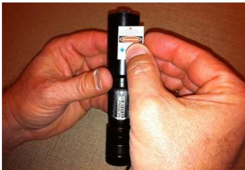
10. Fill out and apply the laser warning label to the heat sink holder, slightly overlapping the battery compartment if necessary. "Max power" is 1,500mW, "Wavelength" is 445nm, "Voltage" is 4.4, "Class" is IV, "Pattern" is Point. **Note:** The red arrowhead on the label points toward the lens. Your laser is now completely assembled and ready for use.
