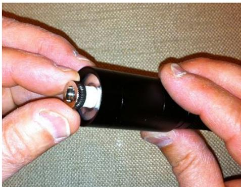
7. Thread the focusing ring/lens assembly about halfway into the diode module. Final adjustment will be completed later. **Reminder:** The **solid slotted end** of the lens assembly faces **away** from the diode. If the lens is installed backwards, the laser dot will have a "bowtie" shape.
