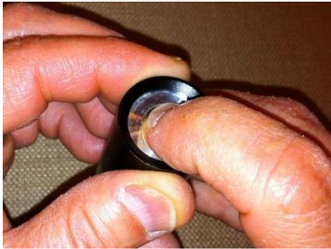
5. Place the bezel/retaining ring over the exposed end of the heat sink. Press the heat sink down with your finger and thread the retaining ring onto the heat sink holder until fully seated. **CAUTION:** Do not touch the diode inside the module with your fingers, and do not let the heat sink rotate as you tighten the bezel/retaining ring. If the heat sink rotates during tightening it could break the wires or pull them off the diode.
