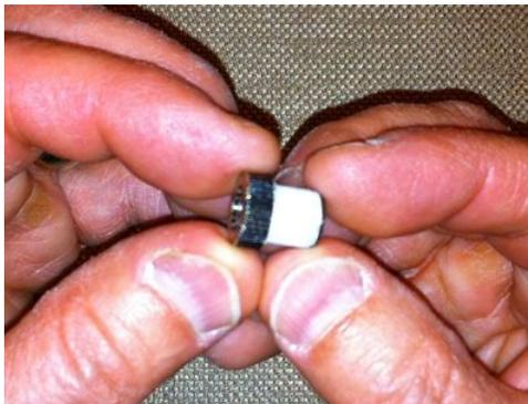
6. If necessary, remove any protective wrapping from the lens assembly. Thread the **solid slotted end** of the glass lens assembly into the lens focusing ring, finger tight. The end of lens assembly with the retaining ring (which may also be slotted) faces the diode. **Note:** for a more snug fit when installing the lens assembly into the diode module, wrap the lens body with a few layers of Teflon tape as shown. **CAUTION:** Do not allow the tape to protrude beyond the end of the lens body.
