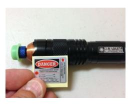
14. Fill out and apply the laser warning label to the heat sink holder, slightly overlapping the battery compartment if necessary. "Max power" is 1,200mW, "Wavelength" is 520nm, "Voltage" is 5, "Class" is IV, and "Pattern" is Point. **Note:** The red arrowhead on the label points toward the lens. Your laser is now completely assembled and ready for use.
