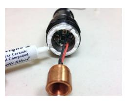
4. Apply a bead of Céramique 2 thermal compound to the narrow annular surface of the driver pill as shown. **CAUTION:** Be careful not to twist or bend the driver leads excessively, and avoid getting the thermal compound on other surfaces.
