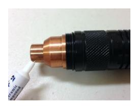
7. Carefully slip the heat sink over the diode module and continue to push it into the heat sink holder until the module protrudes beyond the heat sink and the setscrew hole is barely visible. Apply a thin layer of Céramique 2 thermal compound to the outer surface of the diode module before proceeding with step 8. CAUTION: Do not allow the thermal compound to get in the threaded area inside the diode module.
