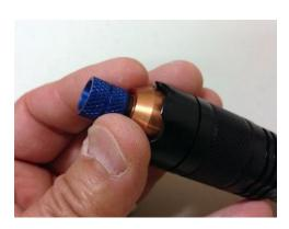
11. Thread the G-2 lens and blue extended focusing ring assembly into the diode module until there is about a 1/16" gap between the bottom of the focusing ring and the diode module. Final focusing adjustment will be completed later. **Note:** If the 'G'-style lens is a snug fit inside the diode module threads, work the lens back and forth a few times in the module to loosen it up a bit.
