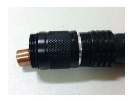
5. Carefully slide the heat sink holder over the diode and driver assembly and thread it onto the battery compartment until fully seated. **CAUTION:** Be careful not to twist or bend the driver leads excessively.
