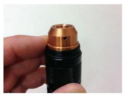
9. Raise the laser assembly to a vertical position and continue to hold the heat sink fully seated in the heat sink holder. The Céramique 2 thermal compound will tend to hold the heat sink in this position against the driver pill due to its "tackiness".
