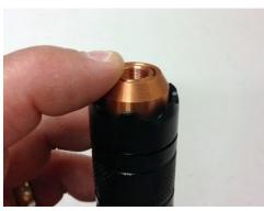
10. Place the bezel/retaining ring over the exposed end of the heat sink. Hold the heat sink down with your finger and thread the retaining ring onto the heat sink holder until fully seated. **CAUTION:** Do not touch the diode inside the module with your fingers, and do not let the heat sink rotate as you tighten the bezel/retaining ring. If the heat sink rotates during tightening it could break the driver wires or pull them off the diode.
