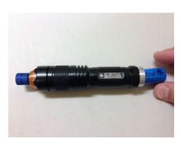
12. WARNING: Beginning at this step put on your protective laser safety goggles and ensure that anyone in the vicinity of your laser is wearing appropriate laser safety goggles. You must assume that your laser will begin functioning as soon as you screw on the tailcap. Install the charged batteries, positive end first, into the battery compartment.
