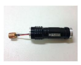
3. **CAUTION:** Remove any static charge on your body by touching a grounded metal object. Place the battery compartment/diode and driver assembly on its side on a stable, flat surface for steps 3 through 8. Thread the diode & driver module into the battery compartment until fully seated. **CAUTION:** Be careful not to twist or bend the driver leads excessively.
