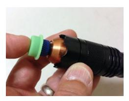
15. Place the lens cap over the lens when your laser is not in use. **CAUTION: Never** operate the laser with the lens cap in place. The cap will burn and combustion residue may be deposited onto the lens surface that can be extremely difficult to remove. **IMPORTANT: DO NOT disassemble the laser once it is assembled.** Doing so may break the wires connecting the driver to the diode and will invalidate your warranty.
