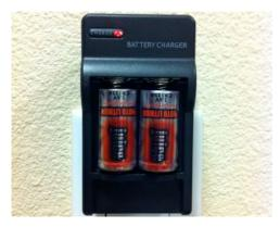
1. Plug in the charger and insert the batteries into the charger in the correct orientation shown in the battery compartments. The light on the charger will glow red until the batteries are fully charged, at which time the light will glow a steady green. Once charged, remove the batteries from the charger. WARNING: Do not attempt to charge disposable batteries in the charger! Note: Charger and/or battery appearance may be different that that shown, blue extended focusing ring shown in photos.
