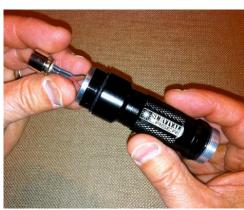
3. **CAUTION:** Remove any static charge on your body by touching a grounded metal object. Thread the diode & driver module into the battery compartment until fully seated. **Be careful not to twist or bend the driver leads excessively.**
