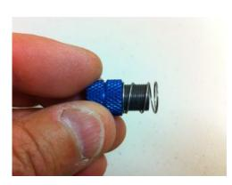
7. Thread the **solid slotted end** of the lens assembly into the extended lens focusing ring, finger tight. Then place the lens spring around the outside of the lens assembly. **Note:** The end of lens assembly with the retaining ring (which may also be slotted) faces the diode.
