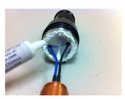
4. Apply a bead of Céramique 2 thermal compound to the narrow annular surface of the driver pill as shown. **CAUTION:** Be careful not to twist or bend the driver leads excessively, and avoid getting the thermal compound on other surfaces.
