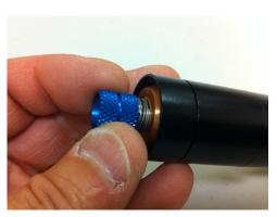
11. Thread the 405-G-1 lens and blue extended focusing ring assembly into the diode module until there is about a 1/16" gap between the bottom of the focusing ring and the diode module. Final focusing adjustment will be completed later. **Note:** The 405-G-1 lens may be a snug fit inside the diode module threads, so you may need to work the lens back and forth a few times in the module to loosen it up a bit.
