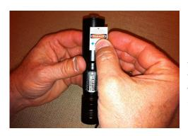
14. Fill out and apply the laser warning label to the heat sink holder, slightly overlapping the battery compartment if necessary. "Max power" is 2,200mW, "Wavelength" is 445nm, "Voltage" is 4.6, "Class" is IV, and "Pattern" is Point. **Note:** The red arrowhead on the label points toward the lens. Your laser is now completely assembled and ready for use.
