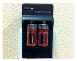
1. Plug in the charger and insert the batteries into the charger in the correct orientation shown in the battery compartments. The light on the charger will glow red until the batteries are fully charged, at which time the light will glow a steady green. Once charged, remove the batteries from the charger. WARNING: Do not attempt to charge disposable batteries in the charger! Note: Charger appearance may be different that that shown.
