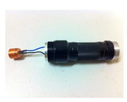
3. **CAUTION:** Remove any static charge on your body by touching a grounded object. Place the battery compartment/diode and driver assembly on its side on a stable, flat surface for steps 3 through 7. Thread the diode & driver module into the batterv compartment until fully seated. **CAUTION:** Be careful not to twist or bend the driver leads excessively.
