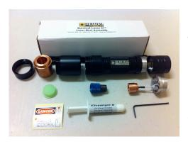
2. Remove and unpack all parts from the laser parts bundle and completely disassemble the laser host into the five major components shown. Verify that all parts are included in the bundle. L-R: bezel/retaining ring, extended copper heat sink w/set screw, heat sink holder, battery compartment, tailcap w/switch and wrist strap, (middle) lens cap, 405-G-1 lens and extended focusing ring assembly, SL II diode & driver (bottom) laser warning label, Céramique 2 syringe, 0.050" Allen wrench.
