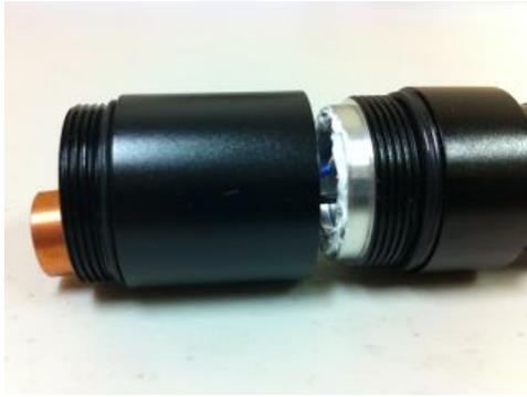
5. Carefully slide the heat sink holder over the diode and driver assembly and thread it onto the battery compartment until fully seated. **CAUTION:** Be careful not to twist or bend the driver leads excessively.
