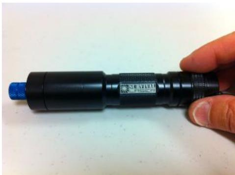
13. Point your laser in a safe direction, away from people, animals and highly flammable or combustible materials. Thread the tailcap w/switch onto the battery compartment until seated. If your laser begins functioning, press the tailcap switch to turn it off.
