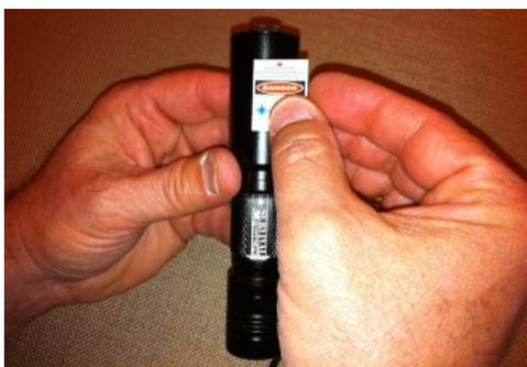
14. Fill out and apply the laser warning label to the heat sink holder, slightly overlapping the battery compartment if necessary. "Max power" is 2,400mW, "Wavelength" is 445nm, "Voltage" is 4.6, "Class" is IV, and "Pattern" is Point. **Note:** The red arrowhead on the label points toward the lens. Your laser is now completely assembled and ready for use.
