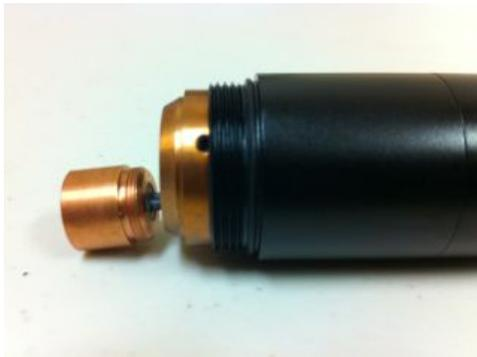
7. Carefully slip the heat sink over the diode module and continue to push it into the heat sink holder until the module protrudes beyond the heat sink and the setscrew hole is barely visible. Apply a thin layer of Céramique 2 thermal compound to the outer surface of the diode module before proceeding with step 8. **CAUTION: Do not allow the thermal compound to get in the threaded area inside the diode module.**
