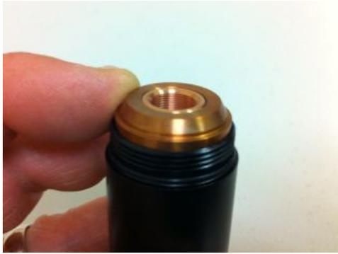
9. Raise the laser assembly to a vertical position and continue to hold the heat sink fully seated in the heat sink holder. The Céramique 2 thermal compound will tend to hold the heat sink in this position against the driver pill due to its "tackiness".
