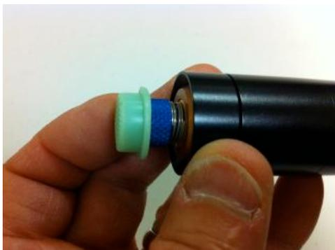
15. Place the lens cap over the lens when your laser is not in use. **CAUTION: Never** operate the laser with the lens cap in place. The cap will burn and combustion residue may be deposited onto the lens surface that can be extremely difficult to remove. **IMPORTANT: DO NOT disassemble the laser once it is assembled.** Doing so may break the wires connecting the driver to the diode and will invalidate your warranty.
