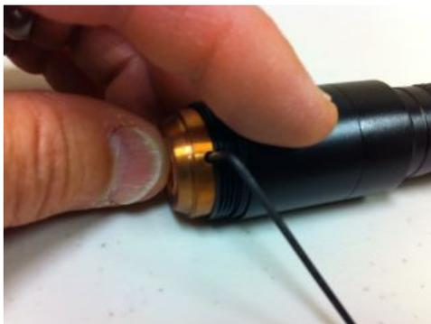
8. Continue to hold the heat sink in this position and push the diode module into the heat sink until the end of the module is flush with the end of the heat sink. Using the 0.050" Allen wrench, **tighten the setscrew securely against the diode module.** Wipe off any excess thermal compound from the module and heat sink. **CAUTION: If the setscrew is not tightened sufficiently, the module could rotate while focusing the lens and break the driver wires or pull them off the diode.**
