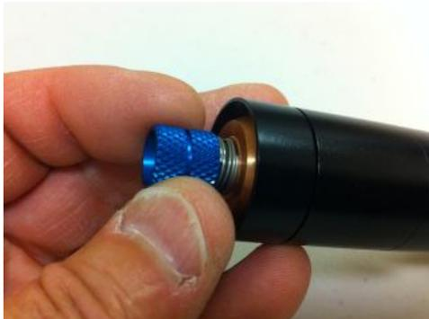
11. Thread the 405-G-1 lens and blue extended focusing ring assembly into the diode module until there is about a 1/16" gap between the bottom of the focusing ring and the diode module. Final focusing adjustment will be completed later. **Note:** The 405-G-1 lens may be a snug fit inside the diode module threads, so you may need to work the lens back and forth a few times in the module to loosen it up a bit.
