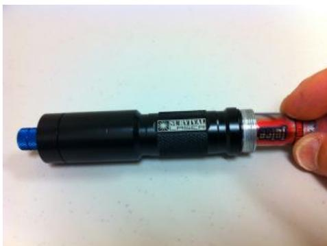
12. **WARNING:** Beginning at this step **put on your protective laser safety goggles and ensure that anyone in the vicinity of your laser is wearing appropriate laser safety goggles.** You must assume that your laser will begin functioning as soon as you screw on the tailcap. Install the charged batteries, **positive end first**, into the battery compartment.
