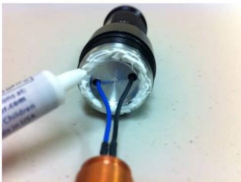
4. Apply a bead of Céramique 2 thermal compound to the narrow annular surface of the driver pill as shown. **CAUTION:** Be careful not to twist or bend the driver leads excessively, and avoid getting the thermal compound on other surfaces.
