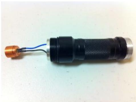
3. **CAUTION:** Remove any static charge on your body by touching a grounded metal object. Place the battery compartment/diode and driver assembly on its side on a stable, flat surface for steps 3 through 7. Thread the diode & driver module into the battery compartment until fully seated. **CAUTION:** Be careful not to twist or bend the driver leads excessively.
