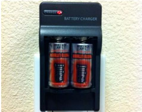
1. Plug in the charger and insert the batteries into the charger in the correct orientation shown in the battery compartments. The light on the charger will glow red until the batteries are fully charged, at which time the light will glow a steady green. Once charged, remove the batteries from the charger. **WARNING: Do not** attempt to charge disposable batteries in the charger! **Note:** Charger and/or battery appearance may be different than that shown.
