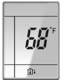
Room Temperature Display
