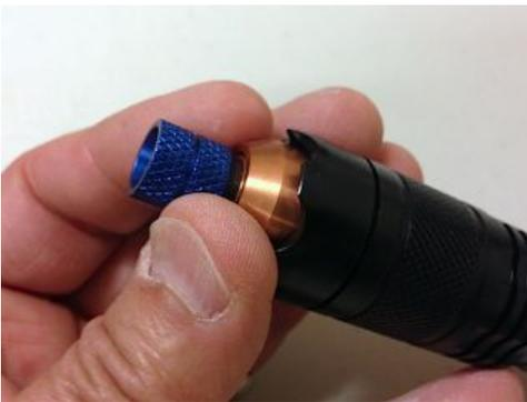
11. Thread the G-2 lens and blue extended focusing ring assembly into the diode module until there is about a 1/16" gap between the bottom of the focusing ring and the diode module. Final focusing adjustment will be completed later. **Note:** If the G-2 lens is a snug fit inside the diode module threads, work the lens back and forth a few times in the module to loosen it up a bit.
