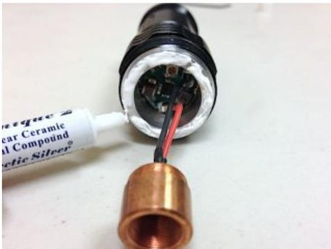
4. Apply a bead of Céramique 2 thermal compound to the narrow annular surface of the driver pill as shown. **CAUTION:** Be careful not to twist or bend the driver leads excessively, and avoid getting the thermal compound on other surfaces. **Note:** The driver controller chip heat sink is not shown in this photo.
