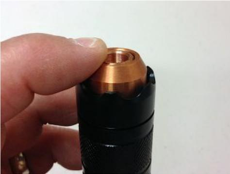
10. Place the bezel/retaining ring over the exposed end of the heat sink. Hold the heat sink down with your finger and thread the retaining ring onto the heat sink holder until fully seated. **CAUTION: Do not** touch the diode inside the module with your fingers, and **do not let the heat sink rotate** as you tighten the bezel/retaining ring. **If the heat sink rotates during tightening it could break the driver wires or pull them off the diode.**
