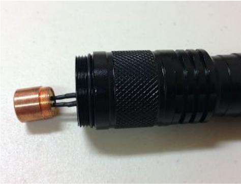
6. (Cont'd) **Note:** There will be some resistance to threading as the battery compartment O-ring is engaged into the heat sink holder during the last two threads.
