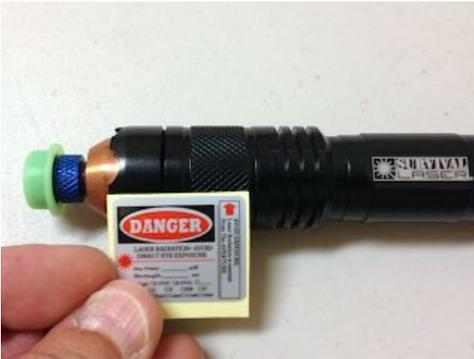
14. Fill out and apply the laser warning label to the heat sink holder, slightly overlapping the battery compartment if necessary. "Max power" is 5,000mW, "Wavelength" is 445nm, "Voltage" is 5, "Class" is IV, and "Pattern" is Point. **Note:** The red arrowhead on the label points toward the lens. Your laser is now completely assembled and ready for use.
