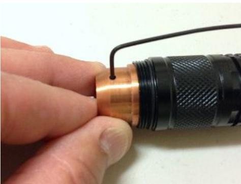
8. Continue to hold the heat sink in this position and push the diode module into the heat sink until the end of the module is flush with the end of the heat sink. Using the 0.050" Allen wrench, **tighten the setscrew securely against the diode module.** Wipe off any excess thermal compound from the module and heat sink. **CAUTION: If the setscrew is not tightened sufficiently, the module could rotate while focusing the lens and break the driver wires or pull them off the diode.**
