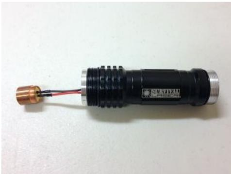
3. **CAUTION:** Remove any static charge on your body by touching a grounded metal object. Place the battery compartment/diode and driver assembly on its side on a stable, flat surface for steps 3 through 8. Thread the diode & driver module into the battery compartment until fully seated. **CAUTION:** Be careful not to twist or bend the driver leads excessively.
