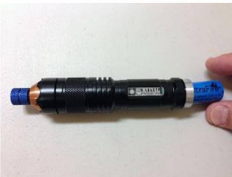
12. **WARNING:** Beginning at this step **put on your protective laser safety goggles and ensure that anyone in the vicinity of your laser is wearing appropriate laser safety goggles.** You must assume that your laser will begin functioning as soon as you screw on the tailcap. Install the charged batteries, **positive end first**, into the battery compartment.
