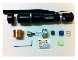
2. Remove and unpack all parts from the laser parts bundle and **completely disassemble the laser host into the five major components shown**. Verify that all parts are included in the bundle. **L-R**: bezel/retaining ring, heat sink holder, battery compartment, tailcap w/switch and wrist strap, heat sink w/set screw, diode & driver module, lens assembly, extended lens focusing ring, external lens spring, 0.050" Allen wrench, laser warning label, silicone lens cap.
