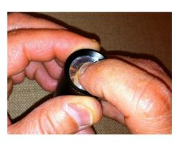
6. Place the bezel/retaining ring over the exposed end of the heat sink. Press the heat sink down with your finger and thread the retaining ring onto the heat sink holder until fully seated. CAUTION: Do not touch the diode inside the module with your fingers, and do not let the heat sink rotate as you tighten the bezel/retaining ring. If the heat sink rotates during tightening it could break the wires or pull them off the diode.
