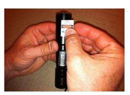
11. Fill out and apply the laser warning label to the heat sink holder, slightly overlapping the battery compartment if necessary. "Max power" is 1,600mW, "Wavelength" is 445nm, "Voltage" is 4.5, "Class" is IV, "Pattern" is Point. **Note:** The red arrowhead on the label points toward the lens. Your laser is now completely assembled and ready for use.
