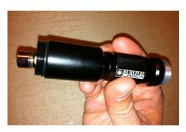
4. Carefully slide the heat sink holder over the driver assembly and thread it onto the battery compartment until fully seated. **Be careful not to twist or bend the driver leads excessively.** There will be some resistance to threading as the battery compartment o-ring is engaged into the heat sink holder during the last two threads.
