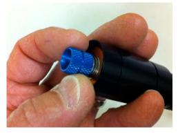
8. Thread the extended focusing ring, lens assembly and lens spring assembled in step 7 about halfway into the diode module. Final focusing adjustment will be completed later. **Reminder:** The **solid slotted end** of the lens assembly faces **away** from the diode. If the lens is installed backwards, the laser dot will have a "bowtie" shape.
