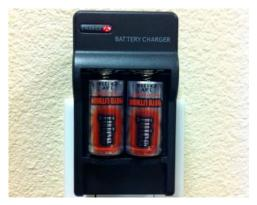
1. Plug in the charger and insert the batteries into the charger in the correct orientation shown in the battery compartments. The light on the charger will glow red until the batteries are fully charged, at which time the light will glow a steady green. Once charged, remove the batteries from the charger. **WARNING: Do not** attempt to charge disposable batteries in the charger! **Note:** Charger appearance may be different that that shown.
