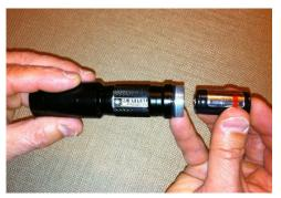
9. **WARNING:** Beginning at this step **put** on your protective laser safety **goggles** and ensure that anyone in the vicinity of your laser is wearing appropriate laser safety goggles. You must assume that your laser will begin functioning as soon as you screw on the tailcap. Install the charged batteries, **positive end first**, into the battery compartment.
